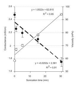
FIGURE 2. Changes in viscosity  $(\circ -)$  and conductance  $(\bullet -)$  of saccharose solutions during sonication.
