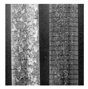
FIGURE 3. Sugar crystals in solutions treated with ultrasounds for 15 min (on the left) and in a control solution after 3 days.
