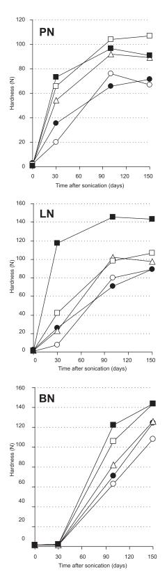
FIGURE 4. Hardness of granulated polyfloral (PN), lime (LN) and buckwheat (BN) honeys after sonication for 0 min ( $\circ$ - $\circ$ ), 3 min ( $\bullet$ - $\bullet$ ), 5 min ( $\Delta$ - $\Delta$ ), 10 min ( $\blacksquare$ - $\blacksquare$ ) and 15 min ( $\square$ - $\square$ ).
